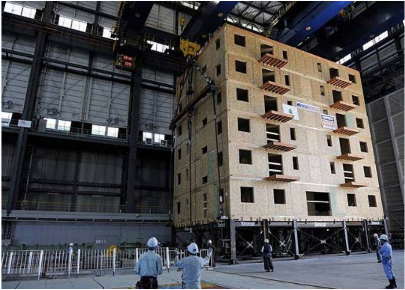
World's largest shake table tests wooden 7 story house's resilience during an earthquake
