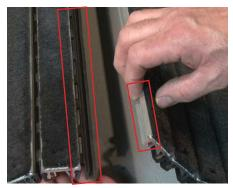
**6** To attach grid modules together, place the foot of the aluminum rail of one module into the rubber connector of the adjacent module.
