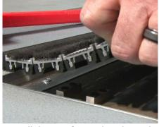
**18** Roll the mat forward so that rails fit snug over locator bars to achieve dimensional fit of the unit.
