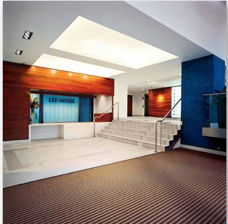
In LEED IEQ Credit 5, the architect/designer is encouraged to specify permanent entryway systems (grilles, grates, etc.) at least 10 ft. in length to capture dirt, water and other particulates at all high volume entryways. This results in improved indoor air quality, reduced maintenance costs and safer floor surfaces that will look beautiful longer.
