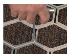
**10** To remove module for cleaning, insert the lift key tool into the drain slot and lift.
