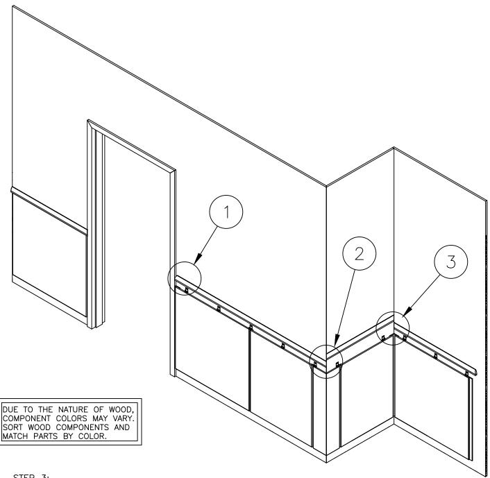
STEP 3: GLUE THE MITERED ENDS AND WAINSCOT TRIM TOGETHER PRIOR TO INSTALLATION. TITEBOND GLUE IS RECOMMENDED FOR THIS APPLICATION.
