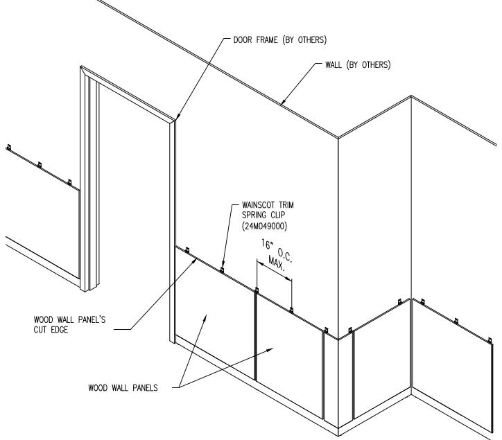
ALL WOOD WALL PANELS SHOULD BE INSTALLED, REFERENCE INSTALLATION INSTRUCTIONS FOR DEMOUNTABLE Z-CLIP WALL PANEL SYSTEM. UPPER HORIZONTAL REVEAL WILL NOT BE NECESSARY BECAUSE WOOD WALL PANEL'S CUT EDGE WILL BE COVERED BY WOOD WAINSCOT TRIM.
