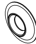
FASTENER #2 #10 COUNTERSUNK FLANGED S/S WASHER (90H047003)
