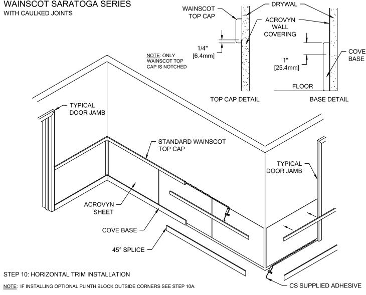
ALL WALL SURFACES MUST BE CLEAN, SMOOTH, DRY AND FREE OF ANY LOOSE PAINT OR ANY OTHER IRREGULARITIES WHICH WOULD PREVENT GOOD ADHESION.
