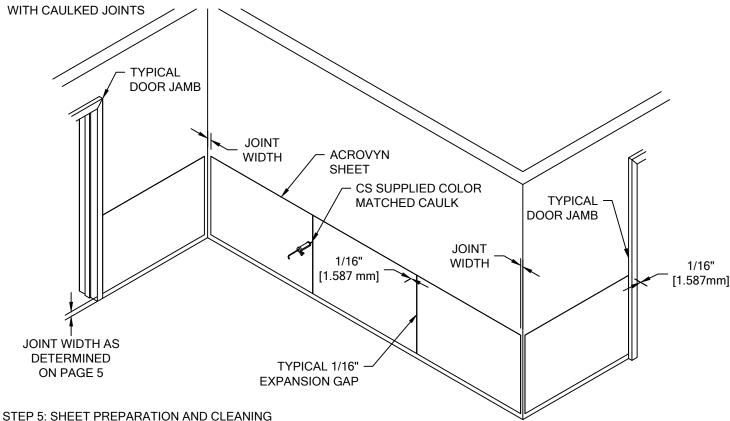
PREPARE THE FIRST SHEET BY MAKING ANY NECESSARY CUTOUTS. REMEMBER TO ALLOW A 1/16" GAP AROUND DOOR AND WINDOW FRAMES, CEILINGS AND BASEBOARDS. USE A STRAIGHT EDGE TO ENSURE NEAT CUTOUTS.
