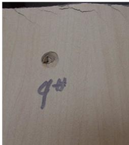
**High Pressure Laminate 4 in lb failure**
