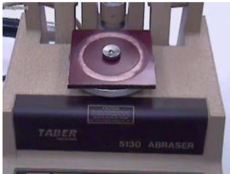
**Wood Veneer w/ Stain and varnish failed sample – 1,000 cycles.**
